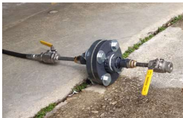
Figure 5. Gasket baseline pressure test rig.
