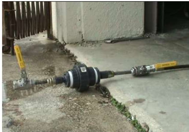
Figure 4. O-ring pressure test rig.
