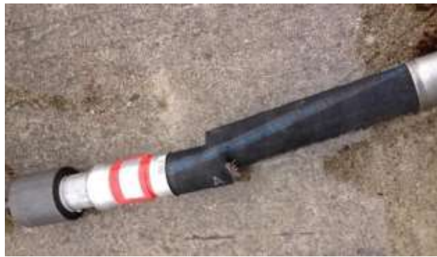
Figure 3. Ruptured HIHTL test specimen.
