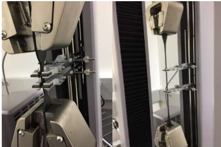
Figure 2. EPDM coupon testing.
